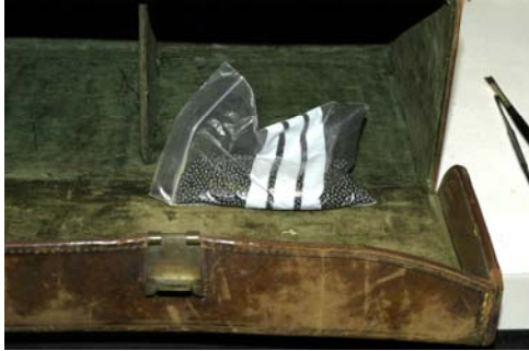
Fig. 11 Bags of lead shot used as weights during adhesion.
