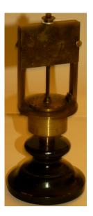
The siren is an instrument invented by Charles Cagniard-Latour in 1819. It was used to determine the number of vibrations in a sound during a determined duration.
