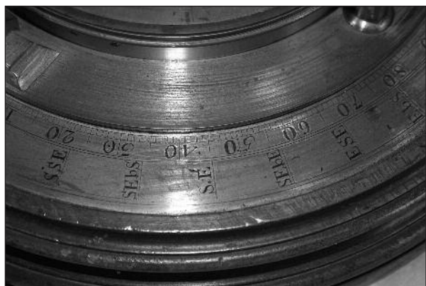
Fig. 3: Base plate of the Rossipher, divided by 10^\circ subdivided to 1^\circ , with 32 compass points. The compass box and the whole mounting are rotated using a pinion working on a hidden rack. (David Bryden, reproduced by permission of Museum of the History of Science, University of Oxford.)
