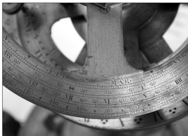
Fig. 6: Ecliptic scale of the Rossipher. A single arrowhead marks 5° intervals. Note that the first point of Aries is at March 9½ indicating that the dial was made for the Julian calendar. Hence the instrument must date from before 1752, the year the Gregorian calendar was introduced into England. (David Bryden, reproduced by permission of Museum of the History of Science, University of Oxford.)
