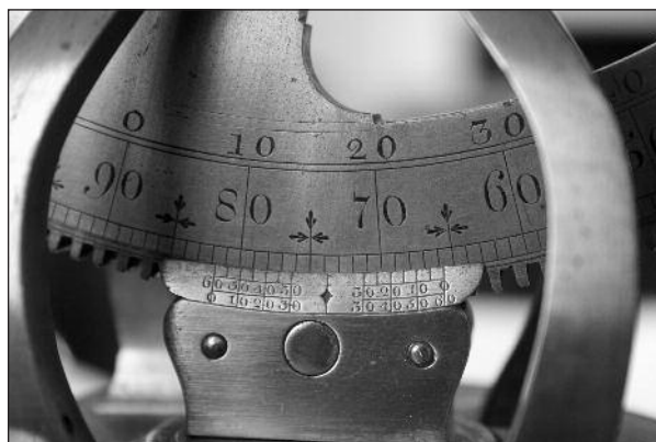
Fig. 4: The vernier read-out on the altitude semicircle, allowing latitudes to be set to the nearest 5 seconds. Note the use of the three arrowheads to mark the 5^\circ interval, and the rack-work on the edge of the circle. (David Bryden, reproduced by permission of Museum of the History of Science, University of Oxford.)
