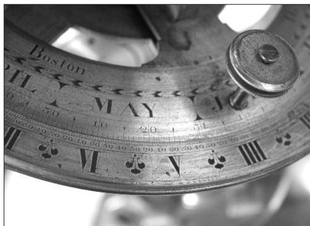
Fig. 5: Equatorial scale of the Rossipher. A fleur-de-lis marks the 30' (half hour?) points and there is a decorative wheat-ear border. Note the knurled-head turnscrew. The rack work is cut on the inside of the hour ring, and hidden by the inner circle of months – this revolves when the pinion is turned via the knurled-head screw. Equivalent times for Boston, Damascus, Fort St George [Madras, India], Pekin, Xalisco [Mexico], and New Severn [Hudson Bay, Canada], can be read on the equatorial hour scale. (David Bryden, reproduced by permission of Museum of the History of Science, University of Oxford.)
