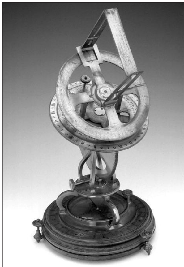
Fig. 1: The Rossipher, the portable universal sundial invented by William Ross. Its base is 270 mm diameter and made of wood, probably walnut. The instrument itself is about half a metre high. (University of Oxford, Museum of the History of Science.)
