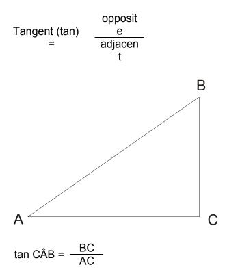
By knowing the base line and the angle CÂB the height BC can be calculated. The Umbra Recta is simply a geometrical trigonometry calculator.
