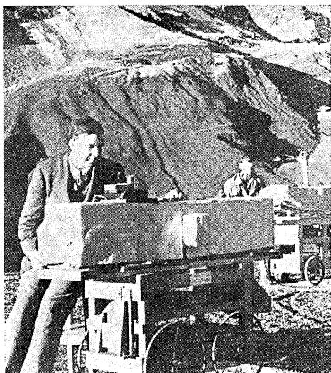
Fig. 11. The first umkehr observations at Arosa in 1932. The instrument on the right (No. 2) operated by A. R. Meetham, is being used for sun observations, while No. 1 is being used for simultaneous observations on the zenith sky.
